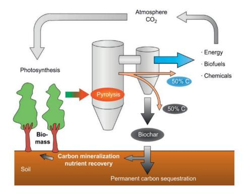
Figure 6: Integrated pyrolysis-based carbon storage and bio-renewables system. Source: (RONSSE; NACHENIUS; PRINS, 2015)
