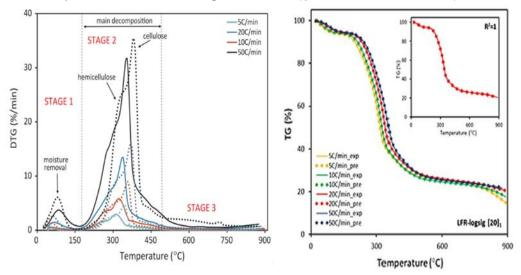
Figure 5: Differential thermal analysis and thermogravimetric analysis of main biomass components at different heating rates. Source: (CEPELIOĞULLAR et al., 2018)
