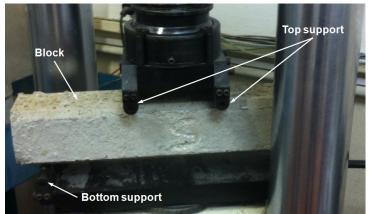
Figure 6 - Positioning of the concrete block for bending test
