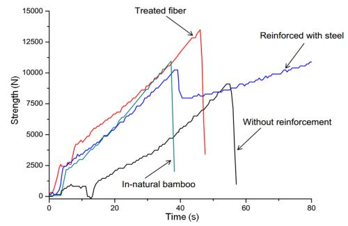
Figure 13 - Curve of the tensile strength on bending test in four point
