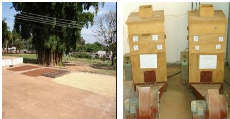
Figure 2 - Drying of natural and washed coffees in yard (left) and fixed bed dryers prototypes (right)
