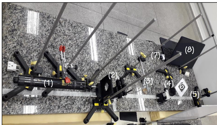
Figure 5- Photograph of the experimental configuration of speckle by reflection: (1) He-Ne laser; (2) Spatial filter; (3) plan-convex lens; (4) Iris; (5) Flat mirror; (6) Sample; (7) Digital Camera; (8) Computer for data processing
