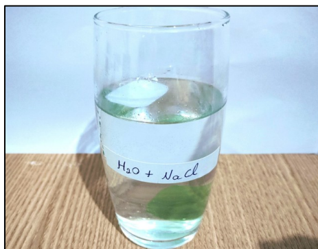
Figure 6 – Polymer samples denser than water in the saltwater solution
