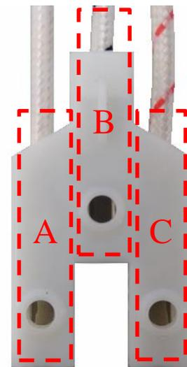
Fig. 2. Electrical connector and its zones: A, B and C.
