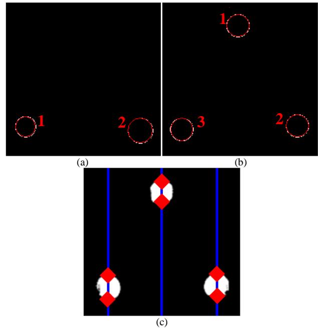
Fig. 9. Resulting images after processing: (a) DSPC detected in zone B by technique  $\alpha$ ; (b) flawless connector processed by technique  $\alpha$ ; (c) flawless connector processed by technique  $\beta$ .
