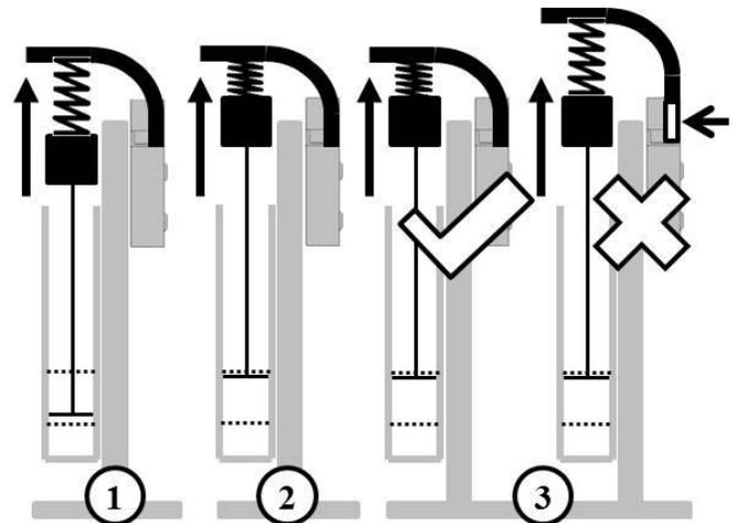
Fig. 5. Schematics of how the test rig works.
