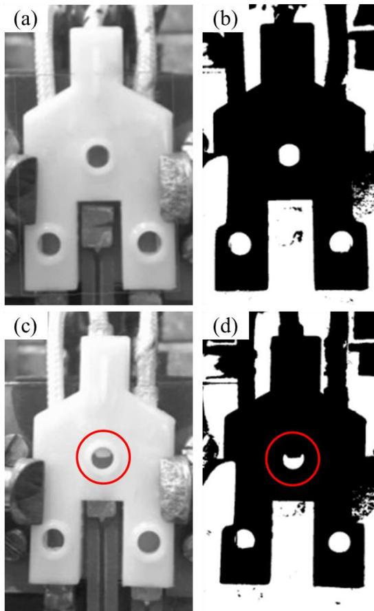
Fig. 8. Comparison of images with and without the defect: (a) electrical connector without defect; (b) thresholding of (a); (c) electrical connector with defect; (d) thresholding of (c).
