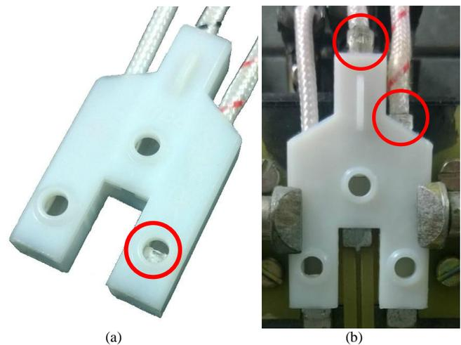
Fig. 3. Electrical connector: (a) DSPC is detectable through the connection openings in zone C and indicated with the red circle; (b) DSPCs are detectable in the upper region of the electrical connector in zones B and C and indicated with the red circles.
