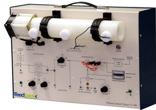
Fig. 6. Front view of the thermal airflow system PT-326.
